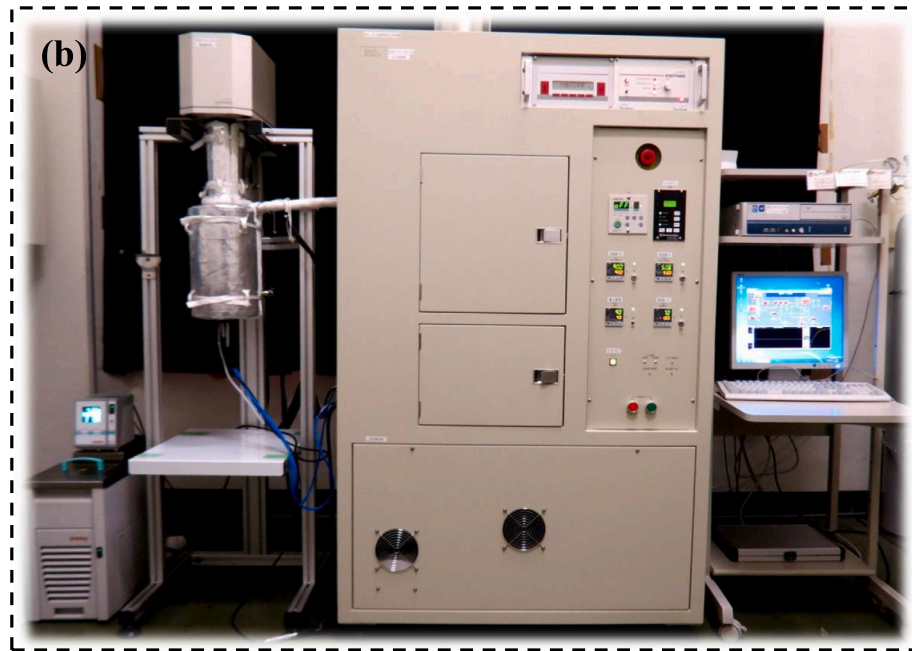
Fig. 2. (a) Schematic diagram and (b) photograph of the experimental apparatus for measuring adsorption isotherms and kinetics of CO 2 onto Maxsorb-III. 1. Magnetic suspension balance; 2. Sample cell; 3. Circulation oil jacket; 4. Oil bath and circulator; 5. Sheathed heater; 6. Refrigerant container; 7. Isothermal oil bath; 8. CO 2 ; 9. Helium; TMP: Turbo-molecular pump; R.P.: Rotary pump; D.P.: Diaphragm pump; T: Thermocouple; P1-P4: Pressure gauges; C1-C2: Controlled valves; V1-V12: Valves.
