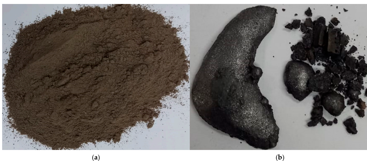
Figure 4. Titanium slag (a), ingot and reduced iron beads (b).
