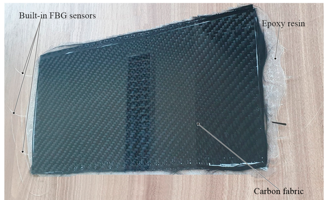
Figure 1. Photograph of a composite carbon fiber and epoxy resin test plate with embedded FBG sensors.
