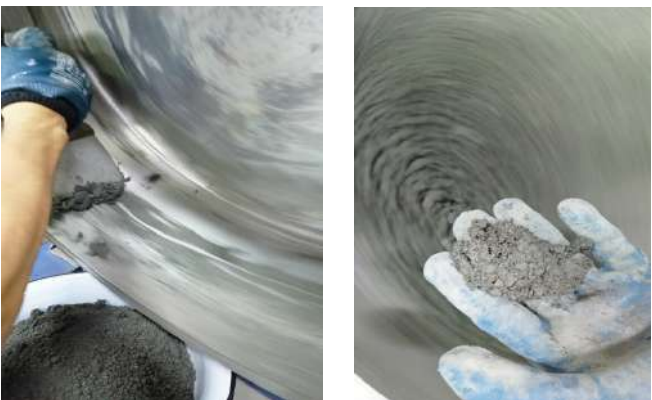
Figure 3: Pelletizing process with PAA and EB binders in the quantity of 1–2 %
