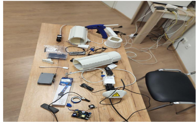
Figure 5: Assembly of a prototype intelligent video surveillance module for a conveyor system.
