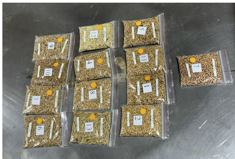
Figure 1. Packaging and arrangement of cereal grain samples for irradiation using the ILU-10 electron beam accelerator.
