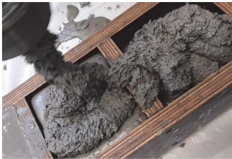
FIGURE 2: Concrete (mortar) samples forming.
