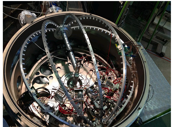
Fig. 1. Scattering chamber of the multi-detector ICARE setup.
