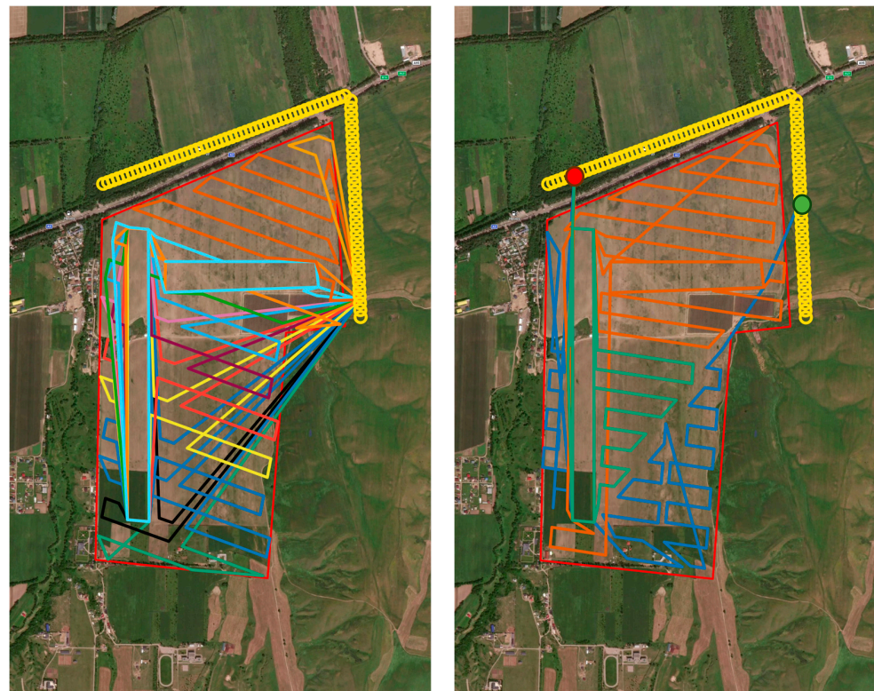
Figure 6. Calculation results for Field 3. (Left) baseline approach, and (right) proposed two-stage method. In the right figure, all drone routes start and end at the same points (marked red circle), except the blue route, which takes off from one location and lands at another (green circle).
