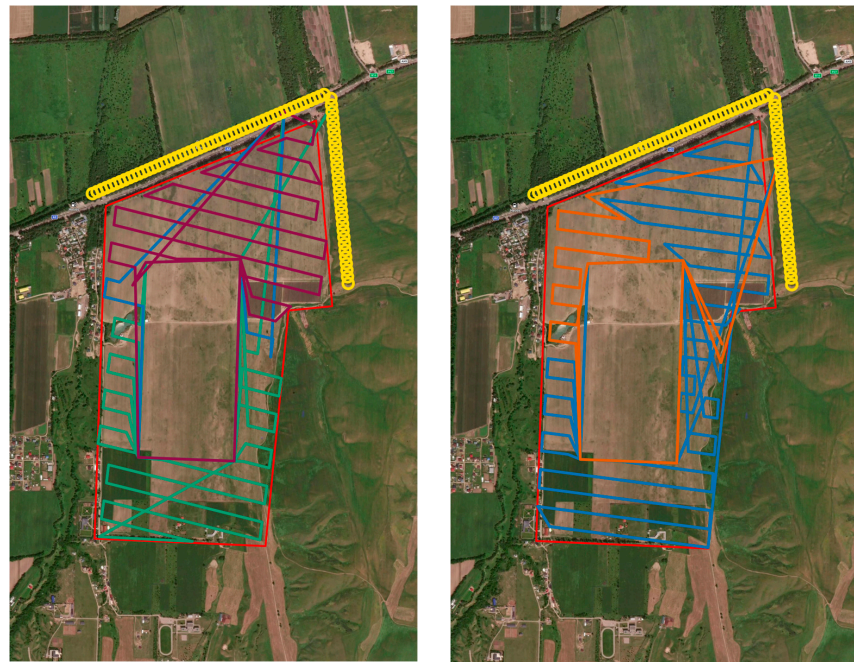
Figure 4. Combined UAV routes for Field 1. ( Left ) baseline approach, and ( right ) proposed two-stage method. The route of the mobile ground support platform is shown by yellow circles.
