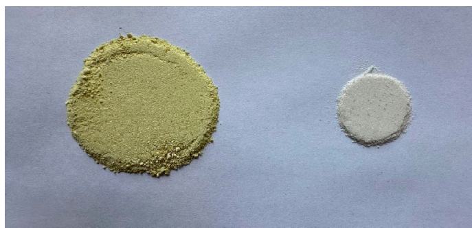
Figure 8. Photographs of solid samples obtained by evaporating tungstic acid solutions at 120^\circ\text{C} : yellow tungstic acid and sodium paratungstate.
