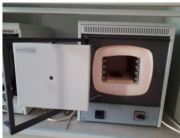
Figure 1. Muffle furnace SNOL-1.4/2.5/1.2–12.5—I1.
