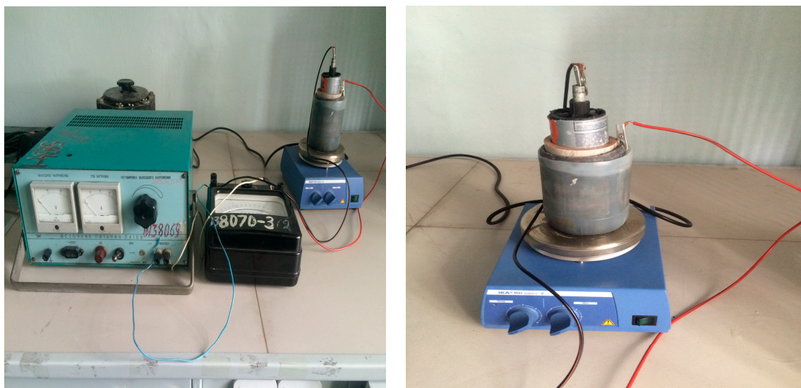
Figure 2. Electrolyzer for electrochemical oxidation of vanadium-containing ores.
