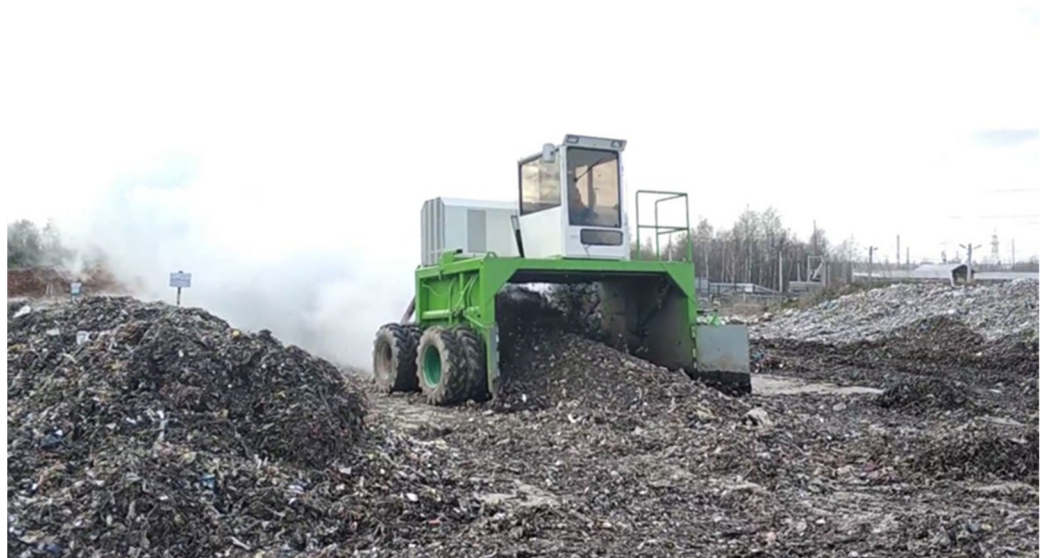
Figure 6. The aeration process of composting ridges facilitated by a turning machine.
