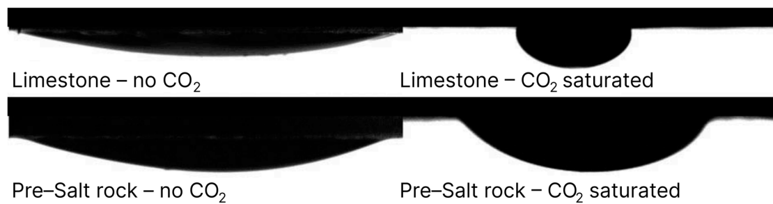
Figure 18. Effect of carbon dioxide on droplet shape and contact angle on limestone surface [65].
