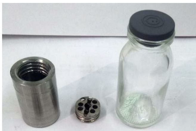
Figure 1. Loading capsule of the ampoule device and investigated samples.
