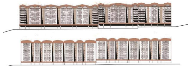
Figure 7 (b). Increasing the area of balconies and installing a superstructure
