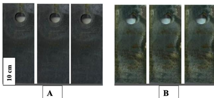
Fig. 3: Appearance of samples with phosphate coatings formed in solution 1 (A) and solution 2 (B) after 8 days of testing in water.
