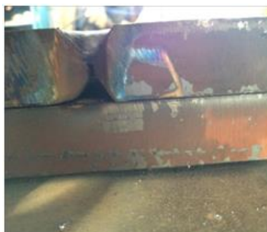
Figure 3 – Welding the surface of a plate made of steel 09G2S with a thickness of 16 mm using the chamfer cutting method
