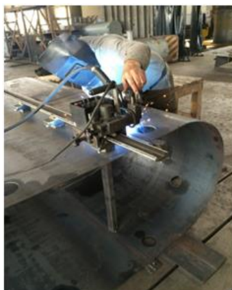
Figure 2 - Welding work in shielding gases
