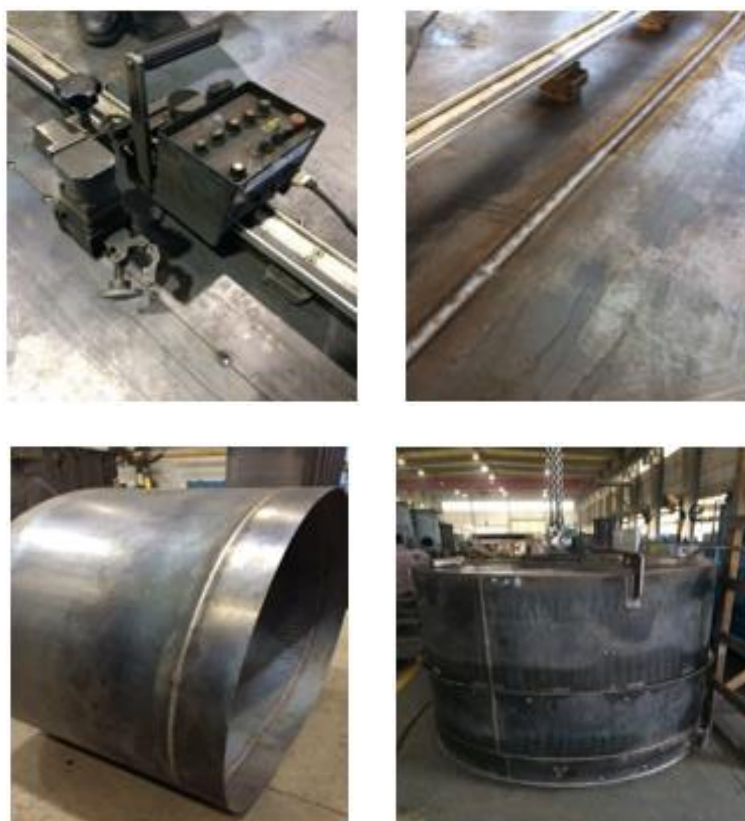
Figure 7 - Capacitance type after welding work
