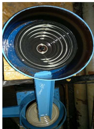
Figure 25. Cascade of vibro-bowl apparatuses, top view.
