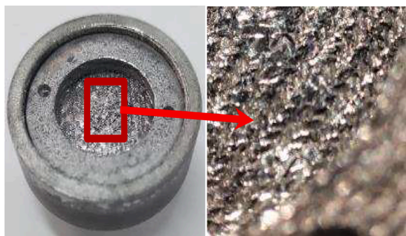
Fig. 4. Fabricated target with Li-Sn CPS.
