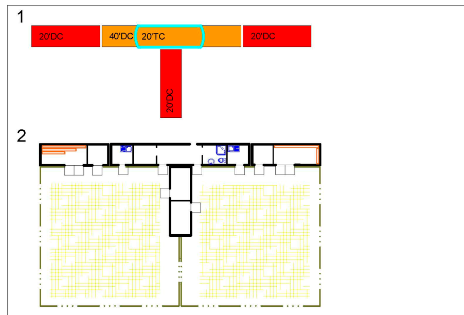
Figure 13. Set 11: 1—The scheme and the kit; 2—the plan of a Display unit for breeding chickens or pheasants. The black lines indicate the constructions of the container; the colored lines indicate the furniture and technological equipment.
