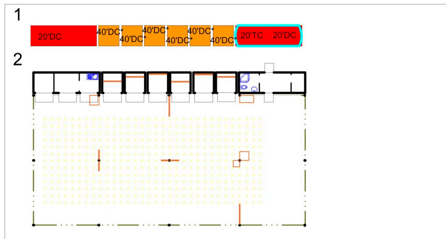
Figure 27. Set 25: 1—The scheme and the kit; 2—the plan of a Display unit for breeding of hunting birds. The black lines indicate the constructions of the container; the colored lines indicate the furniture and technological equipment. The asterisk indicates the vertical position of the container.
