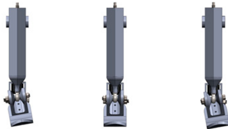
Figure 14. The CAD model shows the ankle–foot prosthesis in three positions: full inversion ( right ), neutral ( center ), and full eversion ( left ).
