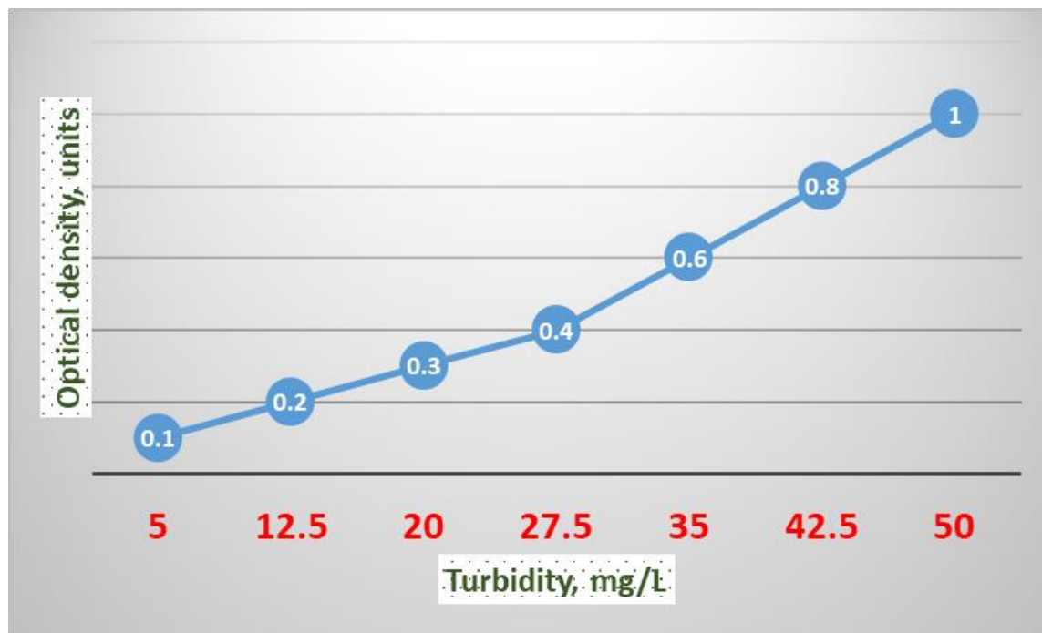
Fig. 10: The variation of density with turbidity.
