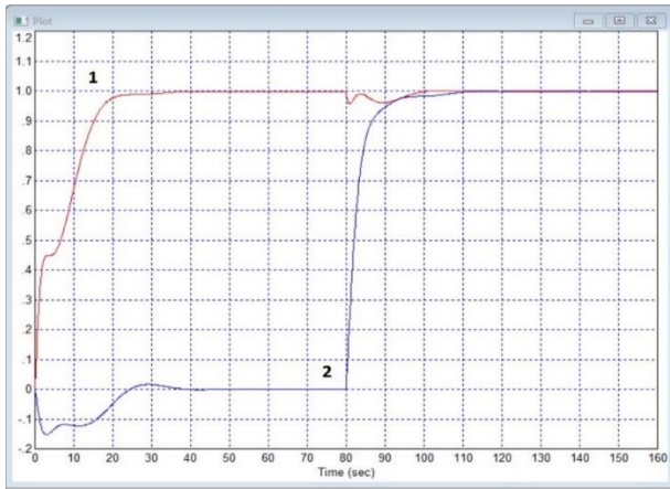
Fig. 2. Transient process in a system with a four-component regulator: 1 - output x_1 , 2 - output x_2
